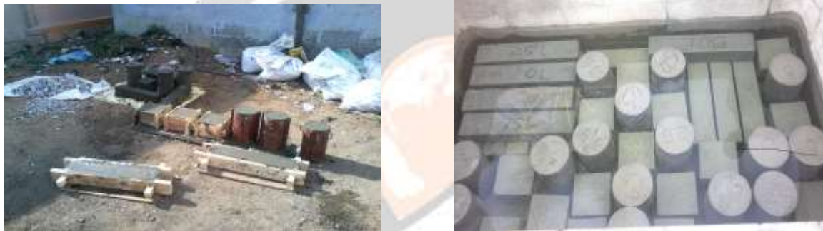
Fig:6 Casting and Curing of concrete specimens
