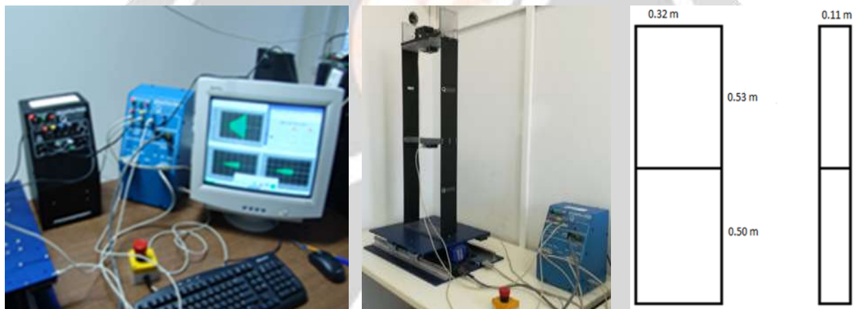
Fig -1: Overview of the shake table and steel structure model
