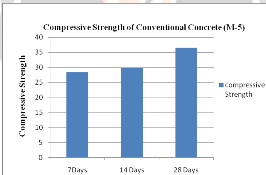
Fig -9: Compressive strength results of M-5 mix
