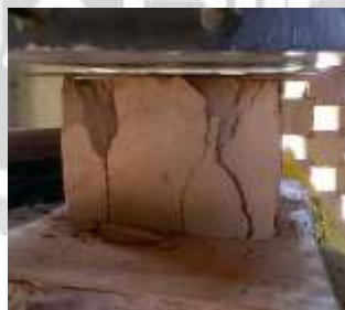
Figure 2: 4 failure of adobe prism
