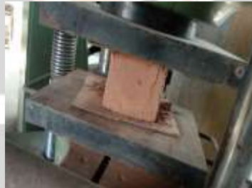
Figure 2: 3 testing of adobe cubes
