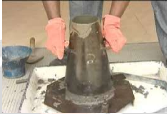
Fig -3.4: Slump Test
