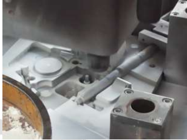
Fig -2 LPDC Bottom Die View with Metallic Core Pin
