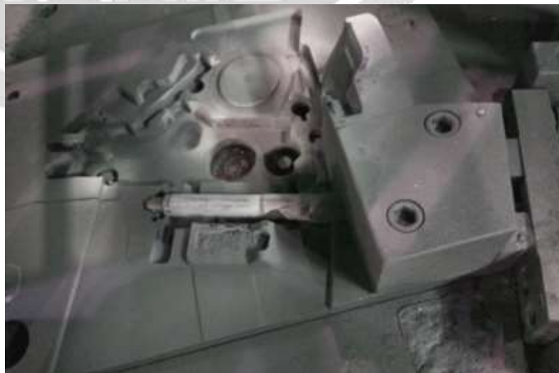
Fig -2 LPDC Bottom Die View with Metallic Core Pin (Bottom)
