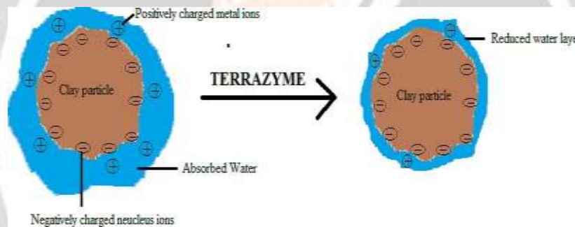
Fig 1 : Mechanism of Terrazyme
