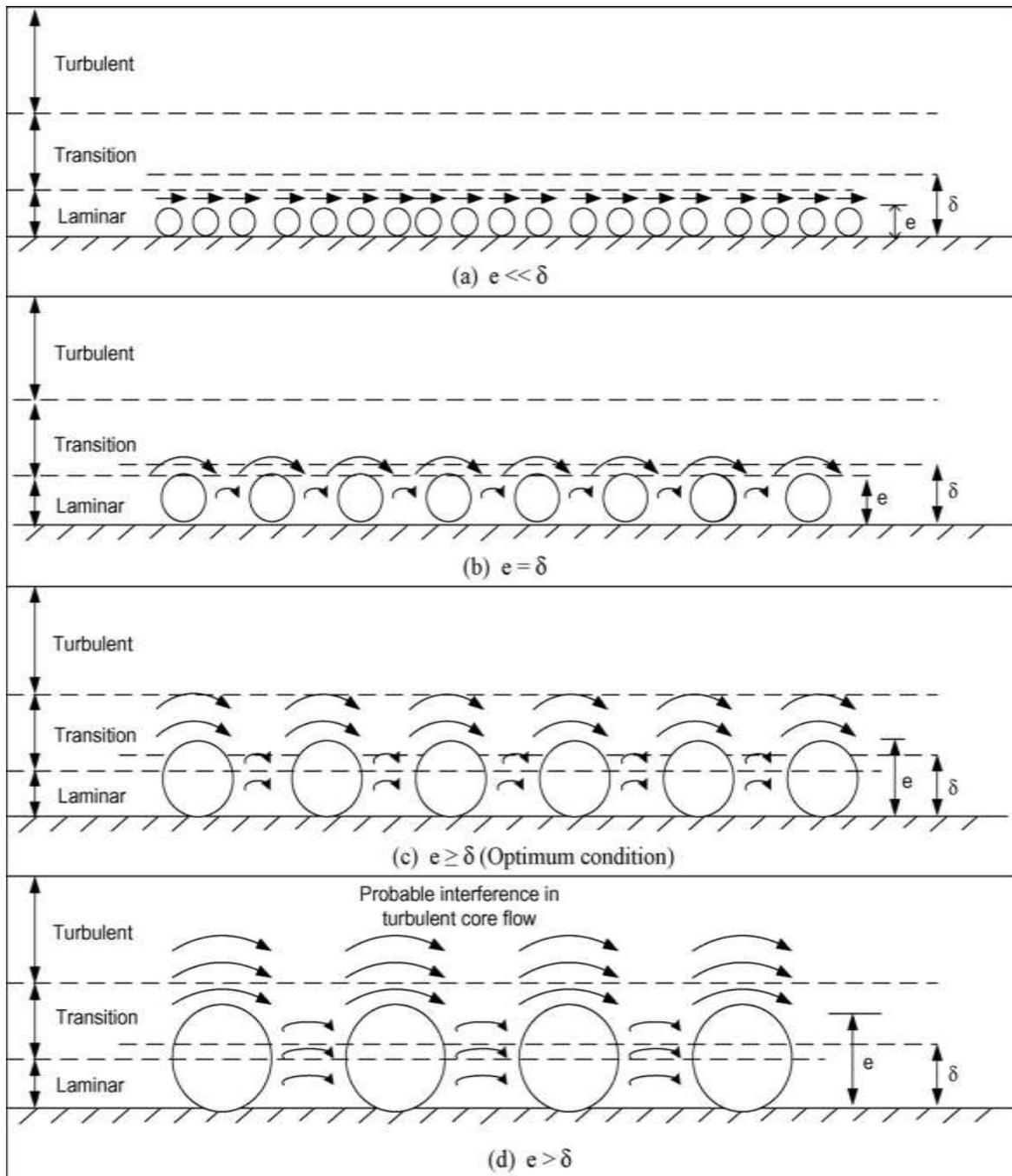
**Fig.1.** Effect of rib height on laminar sub layer
