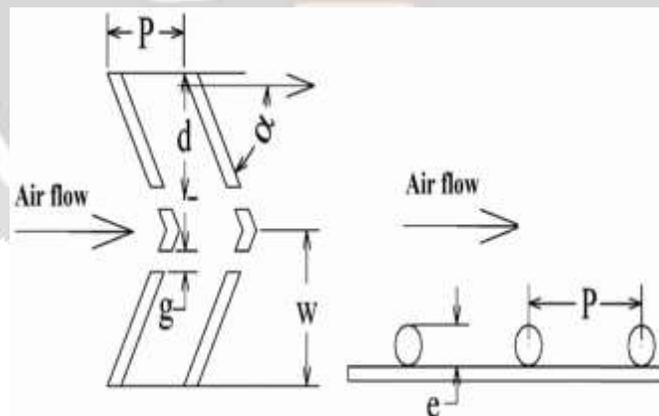
Fig.12. Discrete V- down rib
