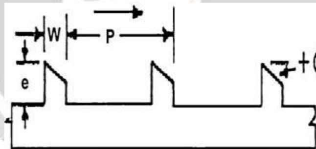
Fig.15. Chamfered ribs
