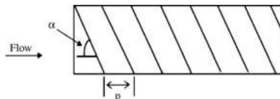
Fig.8. Inclined continuous ribs
