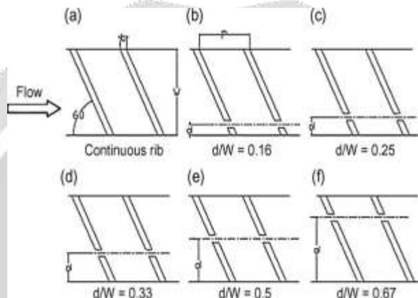
Fig.9 .Inclined rib with gap
