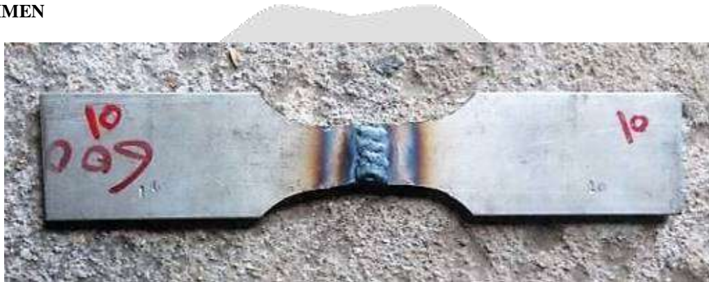
Fig. SPECIMEN SS-304 WITH TIG WELD
