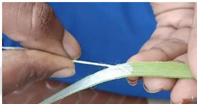
Fig – 1 Extraction of fibres from the bark of the Calotropis gigantea plant
