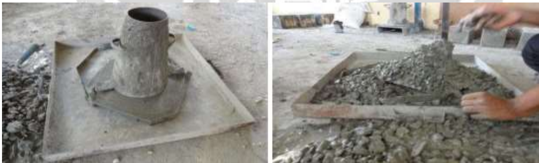
Fig 2 Slump cone and collapse of concrete after lifting
