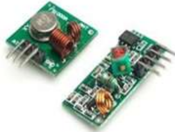
Fig -2: Rf transmitter and Rf receiver
