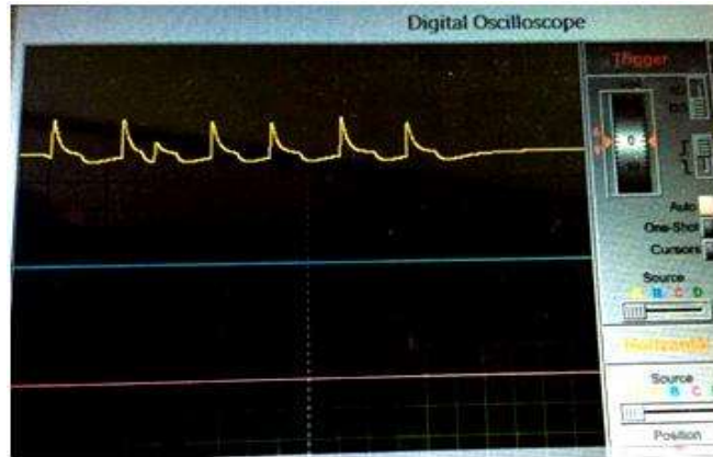
Figure 10- Charging and discharging curve on digital oscilloscope.
