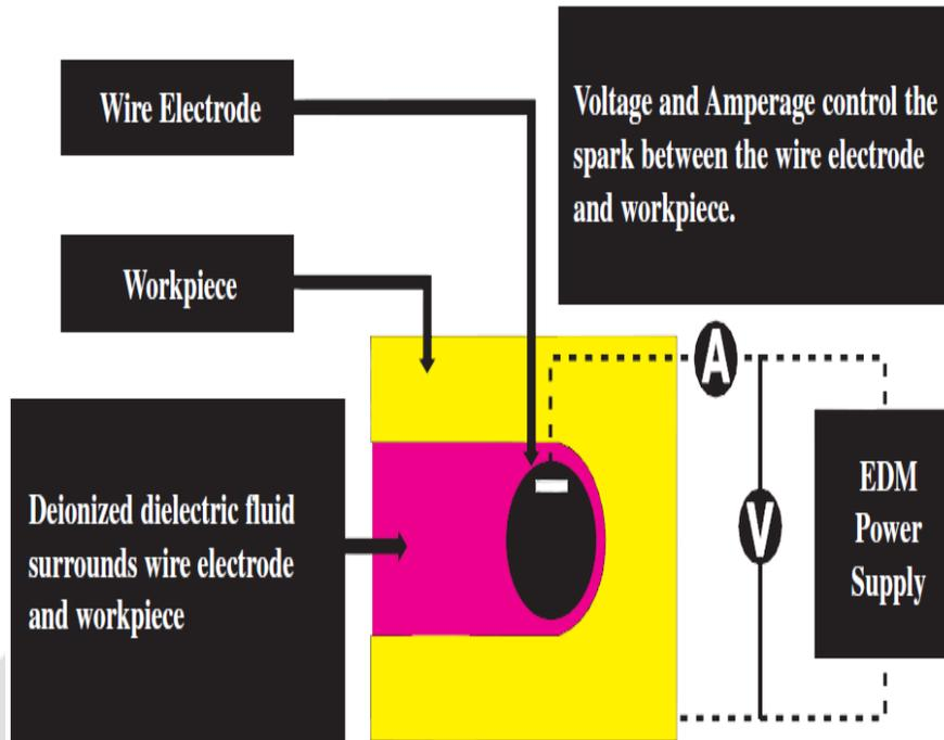
Fig.1.2 WEDM process stage – 1
