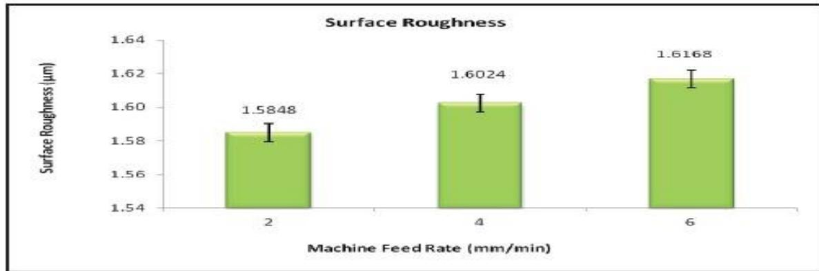
Fig. 2.1 Result on surface roughness at different machine feed
