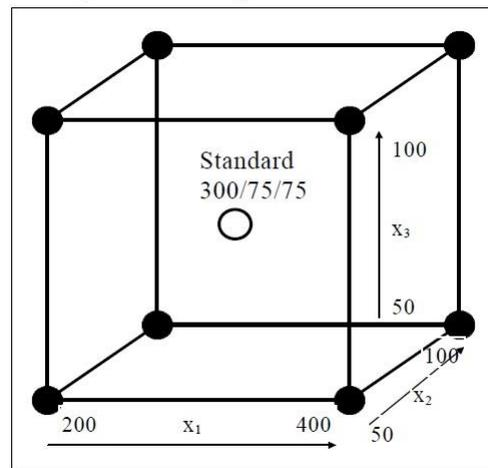
Fig : A symmetrical distribution of experimental points around a center-point experiment.
