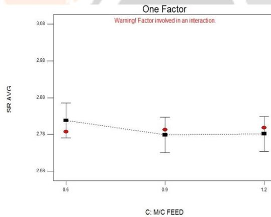
*Fig .MC feed VS SR plot*
