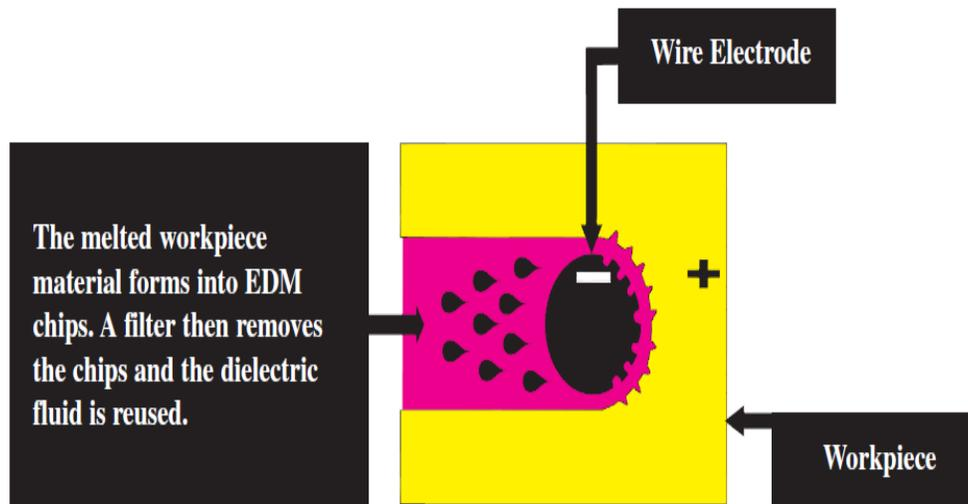
Fig.1.5 WEDM process stage – 4
