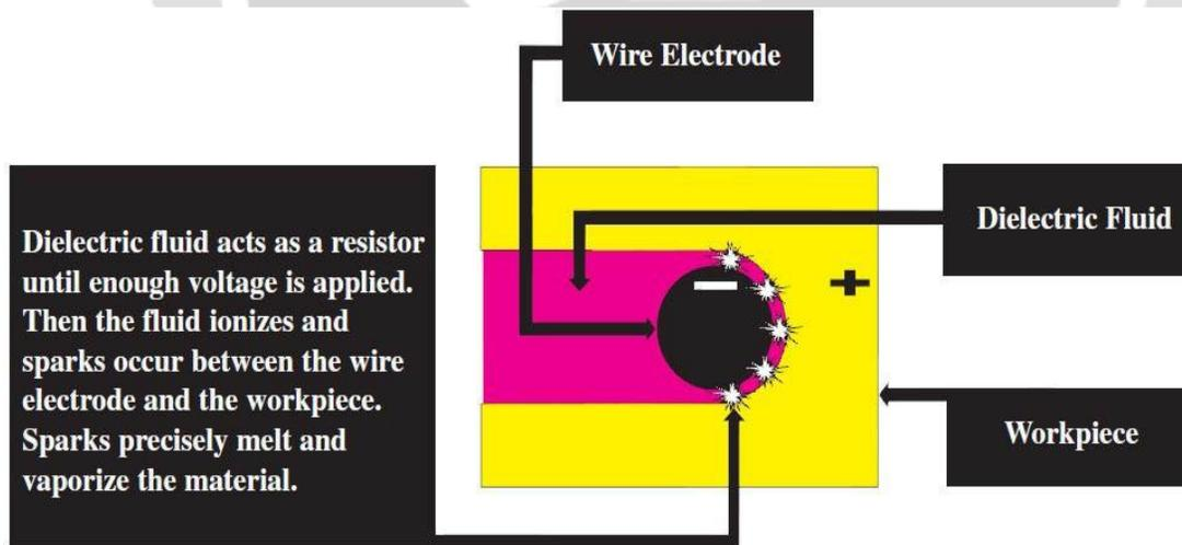
Fig.1.3 WEDM process stage – 2
