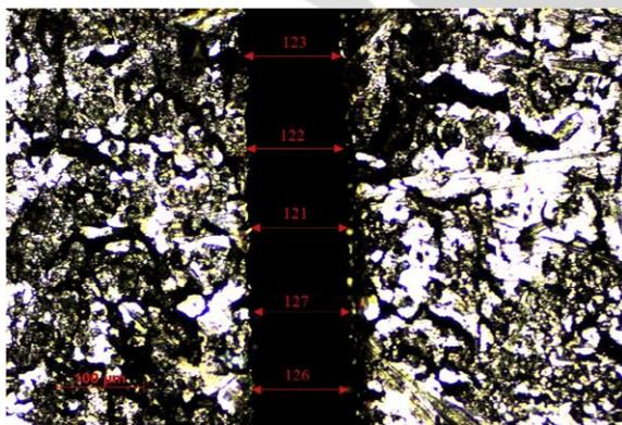
Fig. Kerf width optical measurements in microscope
