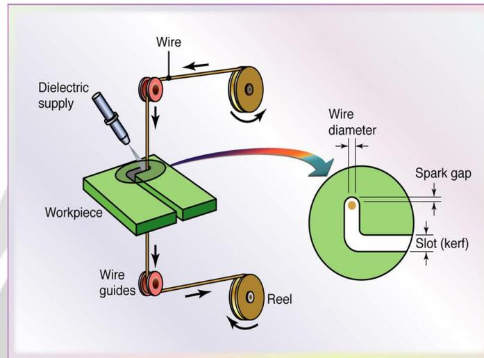
Fig 1.1 wire EDM process
