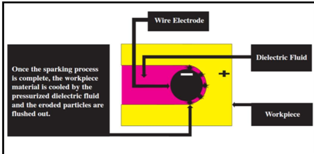
Fig.1.4 WEDM process stage – 3
