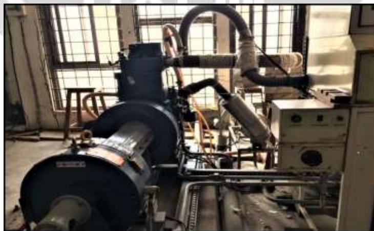
Fig6 : Engine setup with diffuser.
