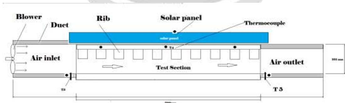
**Fig. 4.1 Schematic diagram of rectangular duct**
