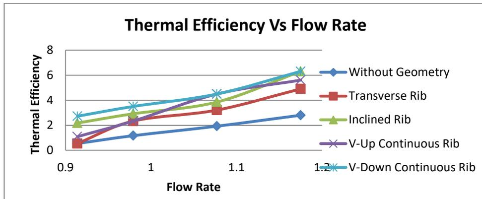
**Fig 1 the variation of the thermal efficiency with flow rate**
