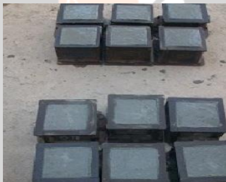
fig -2: casting of concrete cubes.
