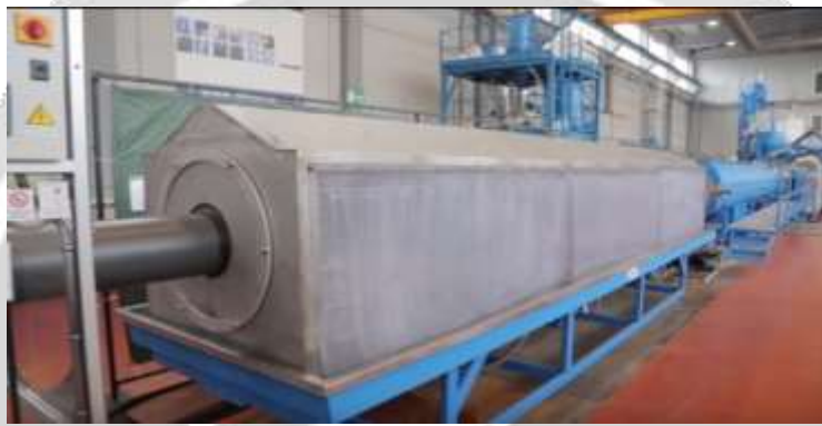
(c) Cooling chambers
