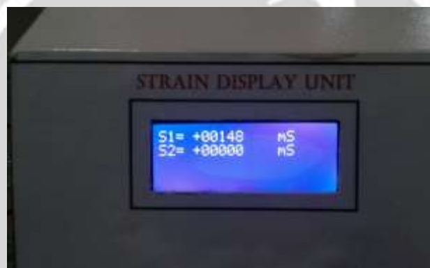
Fig 19. Maximum Principal Strain of Optimized Crane Hook from stain gauge test
