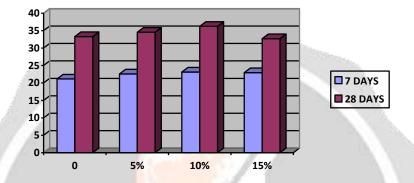
**3.2 Split Tensile Strength:** - Tensile strength of concrete greatly affects the range and size of cracking in concrete. Tensile strength of concrete is less when compared with its compressive strength. Cylinders  $150 \times 300$ mm were used to define the split tensile strength. After curing, the samples were tested on the compression testing machine of 2000kN capacity.
