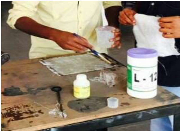
Fig-4. Manual Hand Layup Technique
