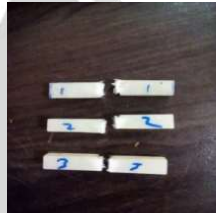
Fig-10: After Impact Testing
