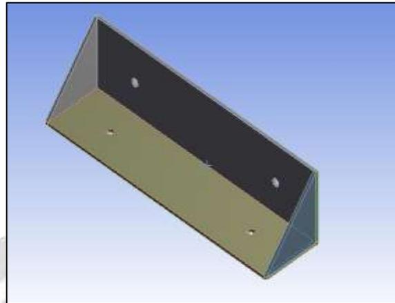
Fig.2.Steel AC mounting bracket
