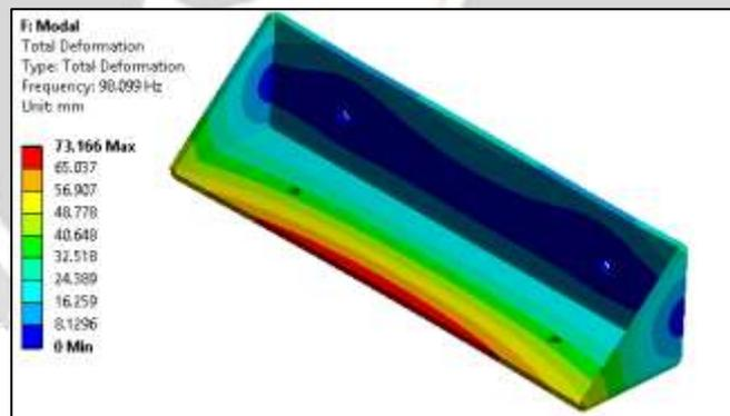
Fig.7.Mode shape plot at 1<sup>st</sup> natural frequency of steel bracket 98.1 Hz
