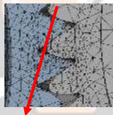
Fig.3 Discretization of CAD model and mesh generation
