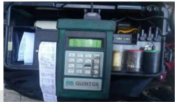
Figure 1.6: Flue gas analyzer
