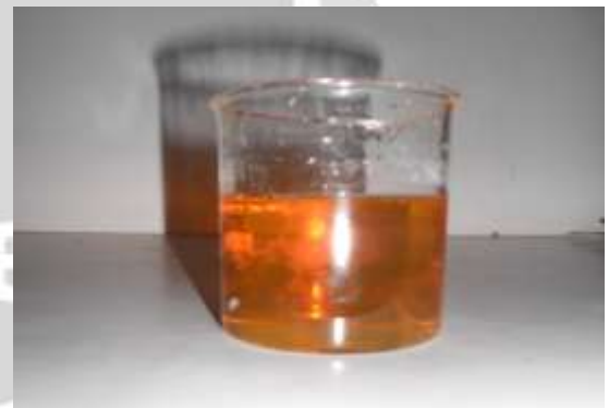
Figure 1.3: Surfactant mixture for emulsion fuel
