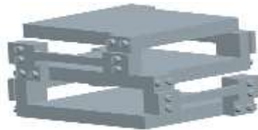
Fig-4: Mechanical Structure of Force Sensor
