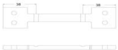
Fig-8 Grooved Beam
