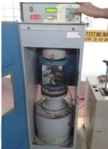
Fig -2: Compressive Strength Testing of Cube
