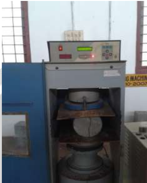
Fig- 3: Split Tensile Testing of cylinder
