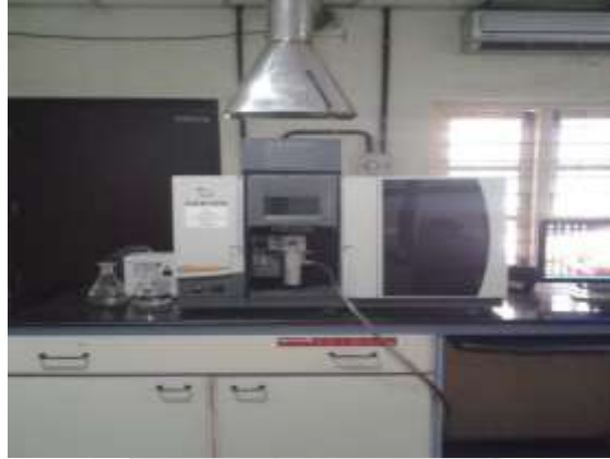
Fig- 1: Atomic Absorption Spectrometer for metal detection
