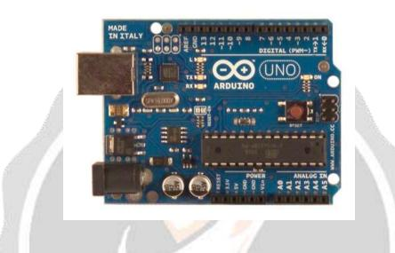
The Arduino Uno is a microcontroller board based on the ATmega328 (datasheet). It has 14 digital input/output pins (of which 6 can be used as PWM outputs), 6 analog inputs, a 16 MHz ceramic resonator, a USB connection, a power jack, an ICSP header, and a reset button. It contains everything needed to support the microcontroller; simply connect it to a computer with a USB cable or power it with a AC-to-DC adapter or battery to get started.
