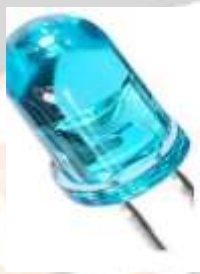
Fig 3.2: Light Emitting Diode
