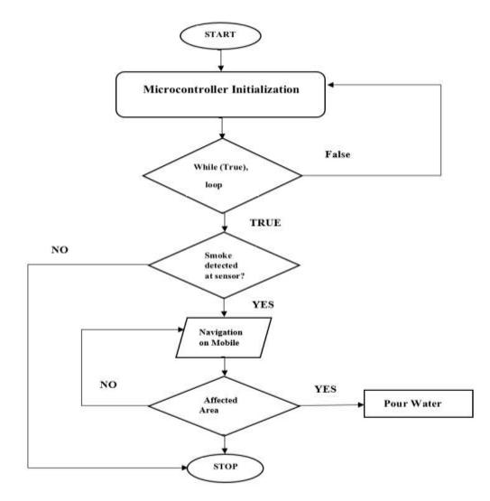
All the process start from mobile application command to microcontroller execution. Smoke detector detects smoke and sends a notification, then mobile application can be used for providing navigation and to sprinkle water on brunt area. It works according to condition that is shown in given flow-chart.
