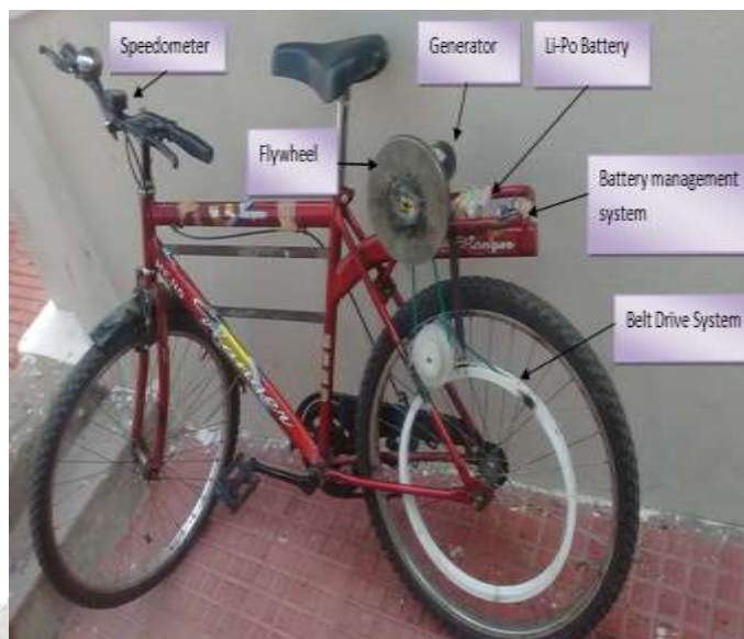
Fig.2: Bicycle generator with a Permanent Magnet Direct Current (PMDC) generator
