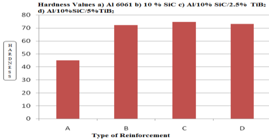
Fig.4-Micro hardness plot of AMC specimens [2]
