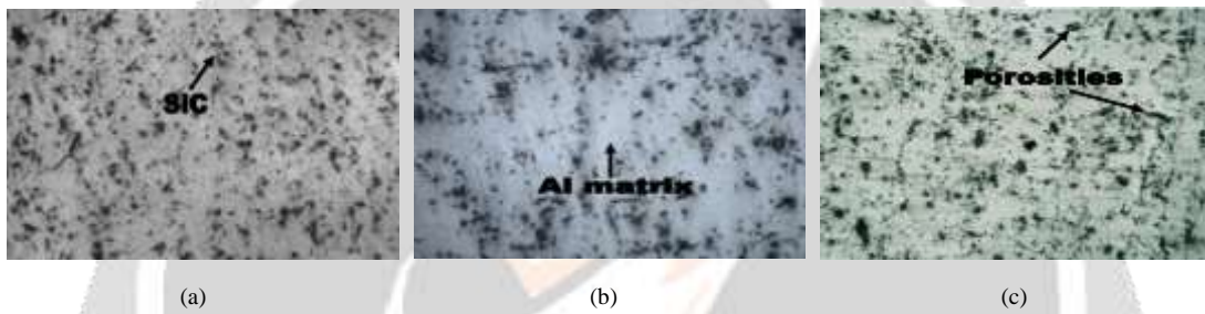
Fig.1 -Microstructures of (a) 5 wt. % (b) 10 wt% (c) 20 wt. % SiC reinforced AMCs [1]
