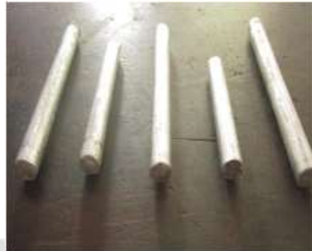
Fig 2.4 Prepared Samples By Using Stir Casting
