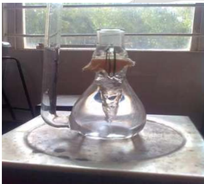
Figure 1.5: Franz diffusion cell with skin mounted between compartments
