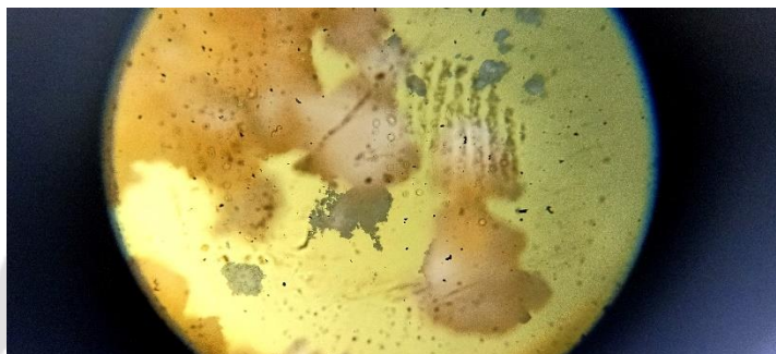
Figure-8: Nimesulide microencapsulation particles in electron microscope
