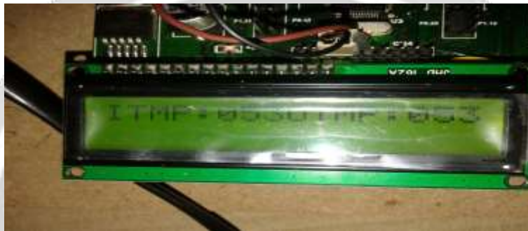
Image 5.2: LCD screen showing Indoor (ITMP) temperature and Outdoor (OTMP) temperature
