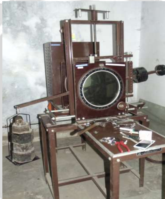
Fig 6.1 Diffused light Polariscopes
