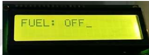
Fig-6: LCD showing fuel off indication
