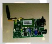
A GSM Modem is a specialized type of modem which accepts a sim card and operates over subscription to a mobile operator, just like a mobile phone. From the mobile operator perspective. The term GSM modem is used as a generic term to refer to any modem that supports one or more of the protocol in the GSM.
