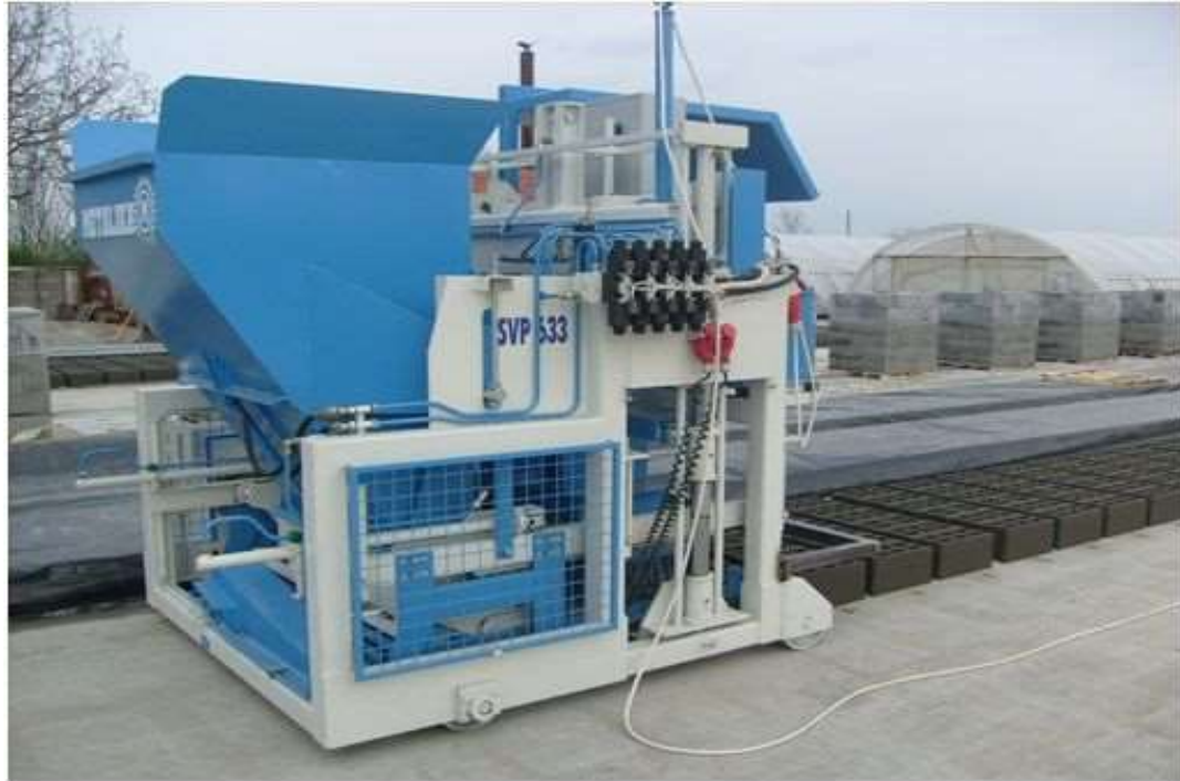
Fig. 2 Movable Concrete Automatic Machine
