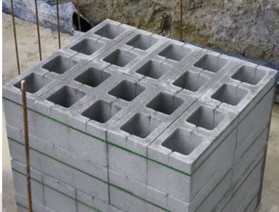
Fig. 7 Block for Load Structure
