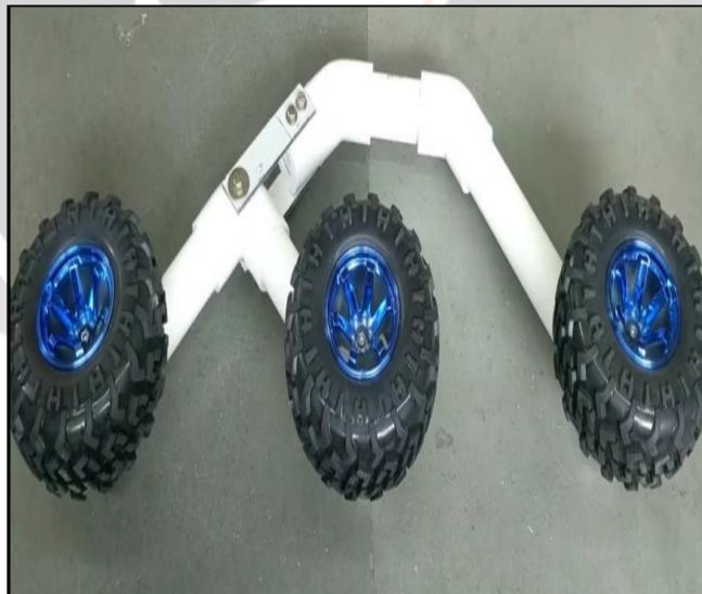
Fig 2. Robotic leg when assembled with wheels
