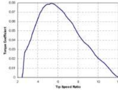
**Fig.1:** Torque coefficient  $C_T$  versus tip-speed ratio  $\lambda$ .
