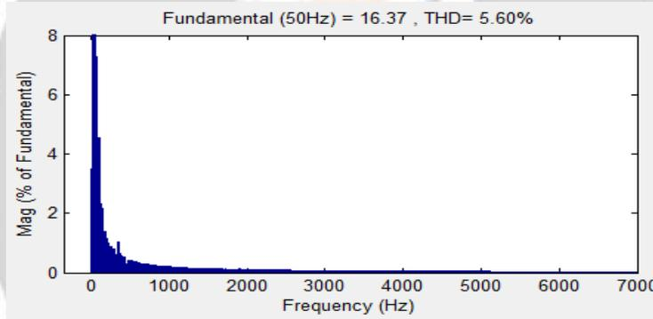
**Fig.11:** Harmonic Content of Inverter Output Voltage
