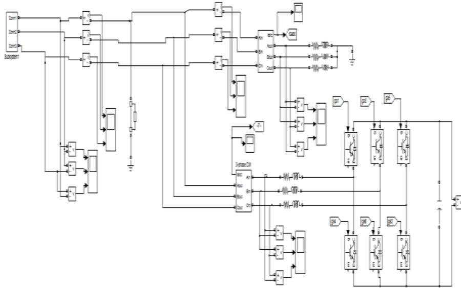
**Fig.6:** Static Compensator at the inverter side
