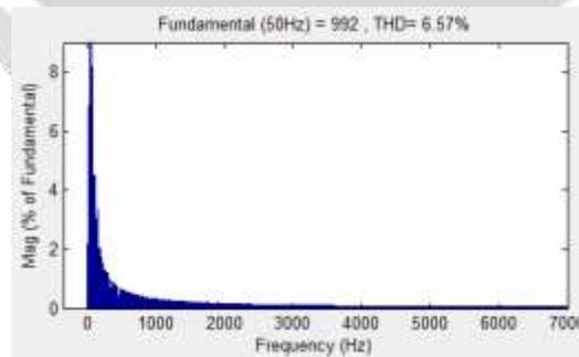
**Fig.12:** Harmonic content of Inverter Output Current
