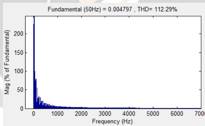
**Fig.5:** Stator Current Harmonics of PMSG
