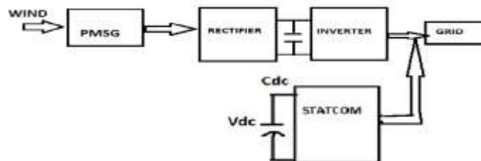
**Fig.2:** Basic Diagram of Wind Energy Conversion system
