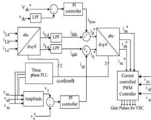
**Fig. 6:** Control algorithm for the three-leg-Voltage Source Converter-based STATCOM
