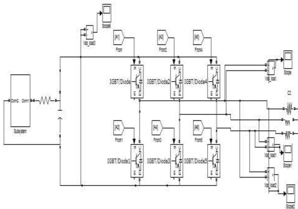
**Fig.4:** Inverter side of the Wind Energy Conversion System
