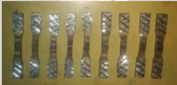
Fig -6: Prepared specimen for tensile test
