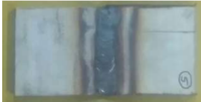
Fig -4: Welded specimen of size 50×100×6 mm
