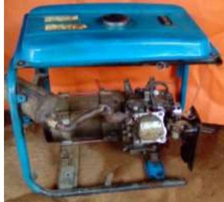
Fig -3: The single-cylinder spark-ignition engine studied
