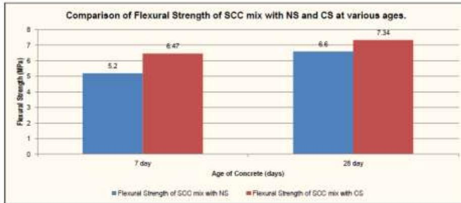
**Fig. 2.2c: Variation in the Flexural Strength of the SCC mixes with NS & CS at various ages**
