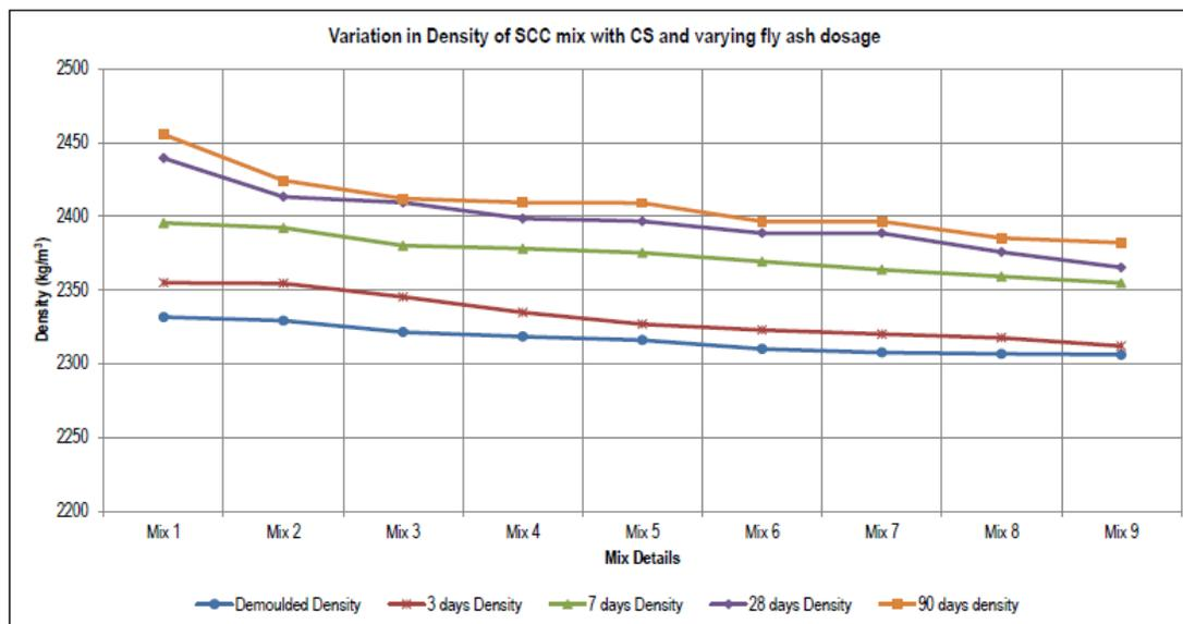
**Fig. 2.4: Variation in density for SCC mix with CS and varying fly ash dosage**
