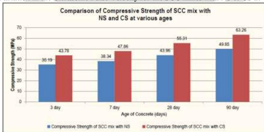
Fig 2.2d: Variation in the Compressive Strength of the SCC mixes with NS & CS at various ages
