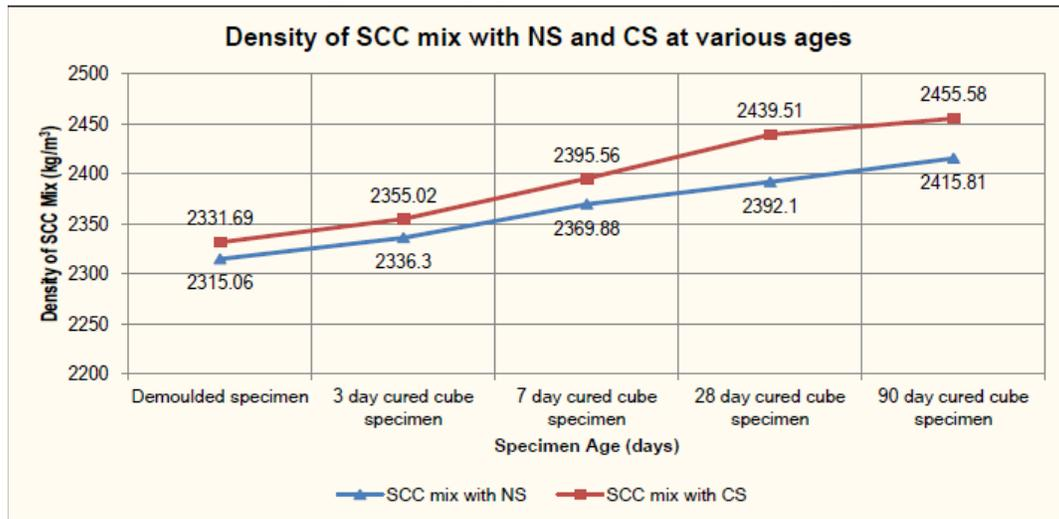
**Fig. 2.2a: Variation in the density of the SCC mixes with NS & CS at various ages**
