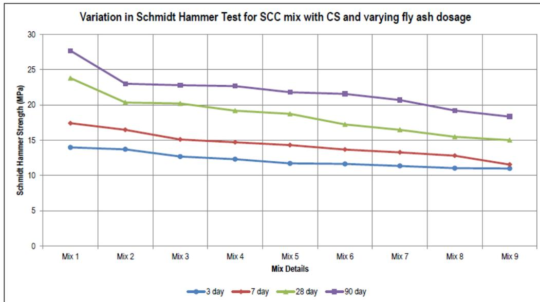
**Fig. 2.5: Variation in Schmidt Hammer Test for SCC mix with CS and varying fly ash dosage**
