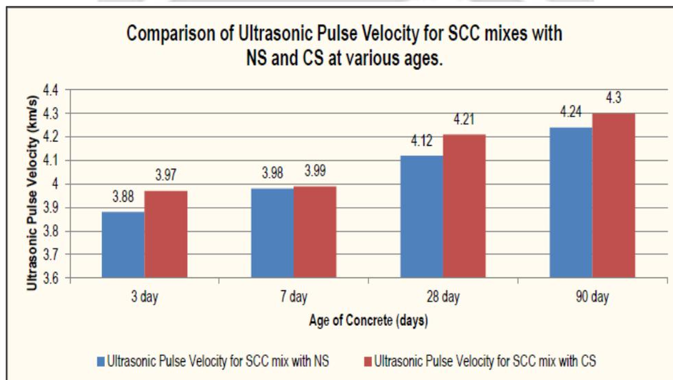
Fig. 4.2c: Variation in the Ultrasonic Pulse Velocity for the SCC mixes with NS & CS at various ages
