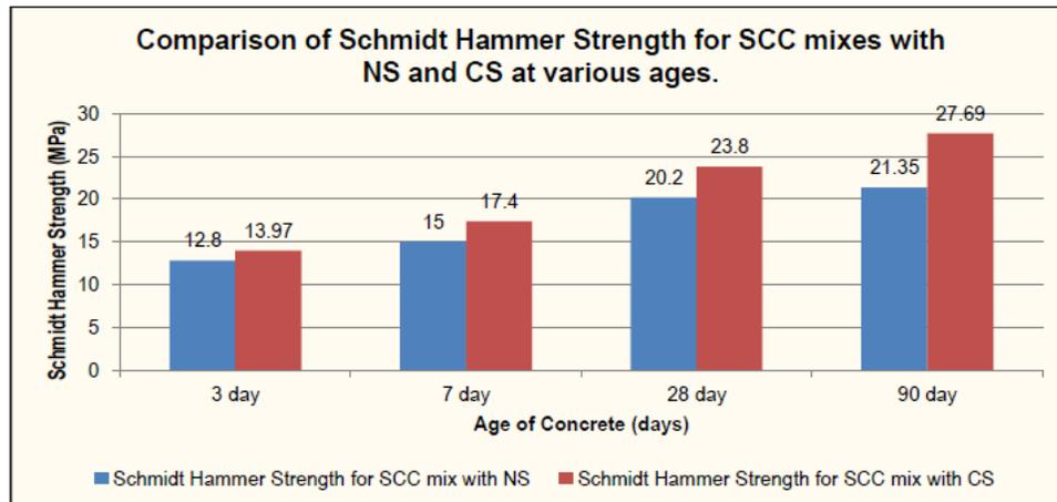
Fig. 2.2b: Variation in the Schmidt Hammer Strength for the SCC mixes with NS & CS at various ages
