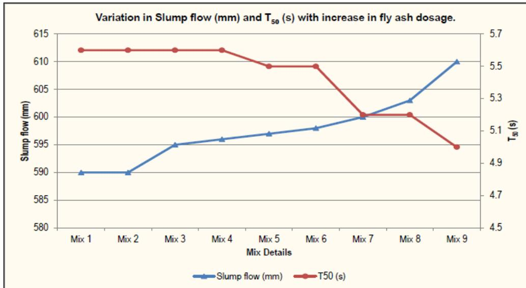
**Fig. 2.3: Variation in slump flow and T50 time for SCC mix with CS and varying fly ash dosage**
