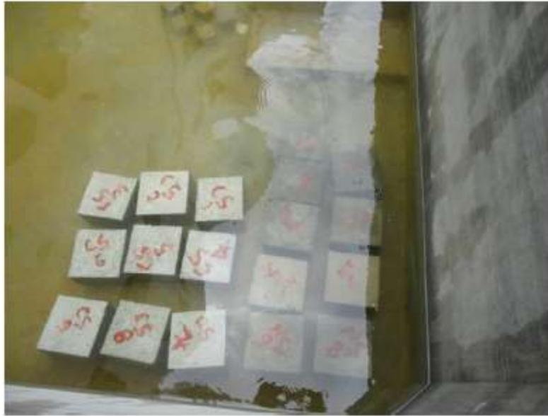
**Fig. 2.1: Curing of SCC mix specimens**
