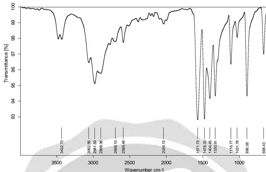
**Figure 3** The FTIR spectrum of LMC crystal
