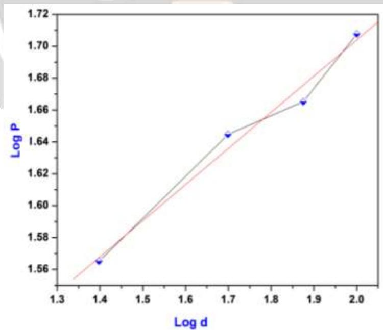
Figure 8 plot of  $\log d$  versus  $\log p$  of LMC crystal
