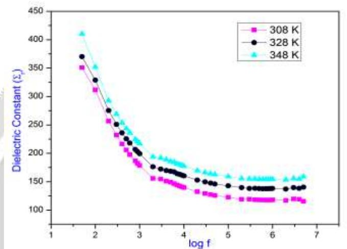
**Figure 5** Variation of dielectric constant with log frequency at different temperatures for LMC crystal
