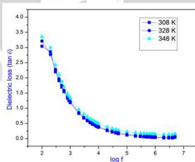
**Figure 6** Variation of dielectric loss with log frequency at different temperatures for LMC crystal
