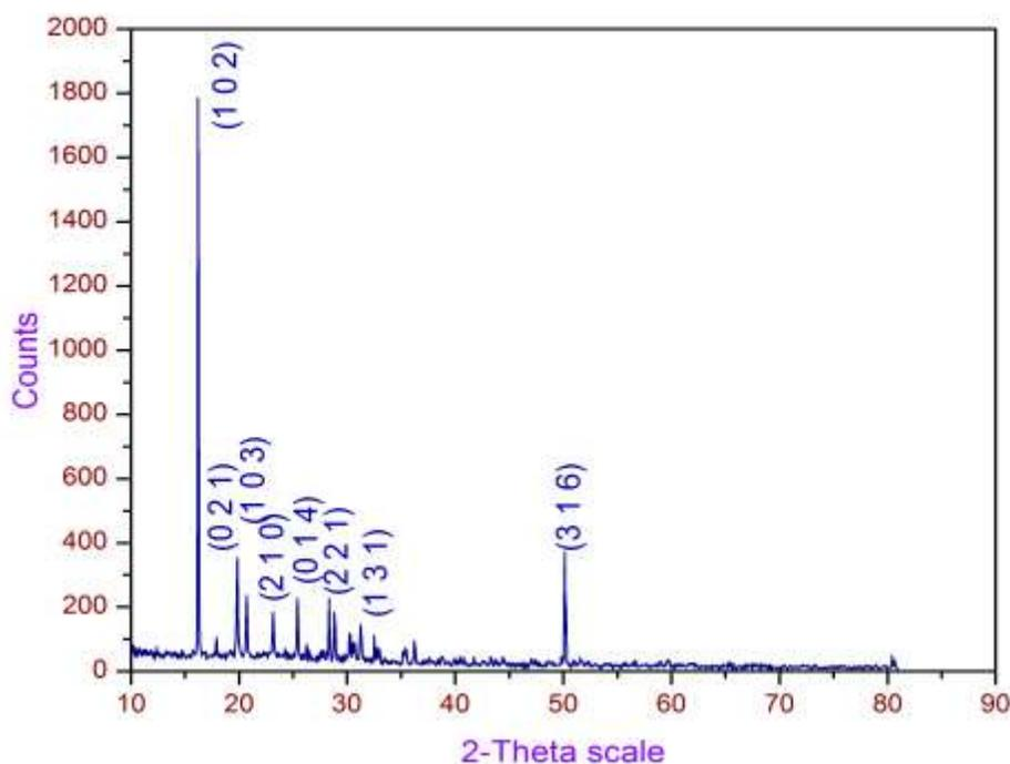
Figure 2 The powder XRD pattern of LMC crystal
