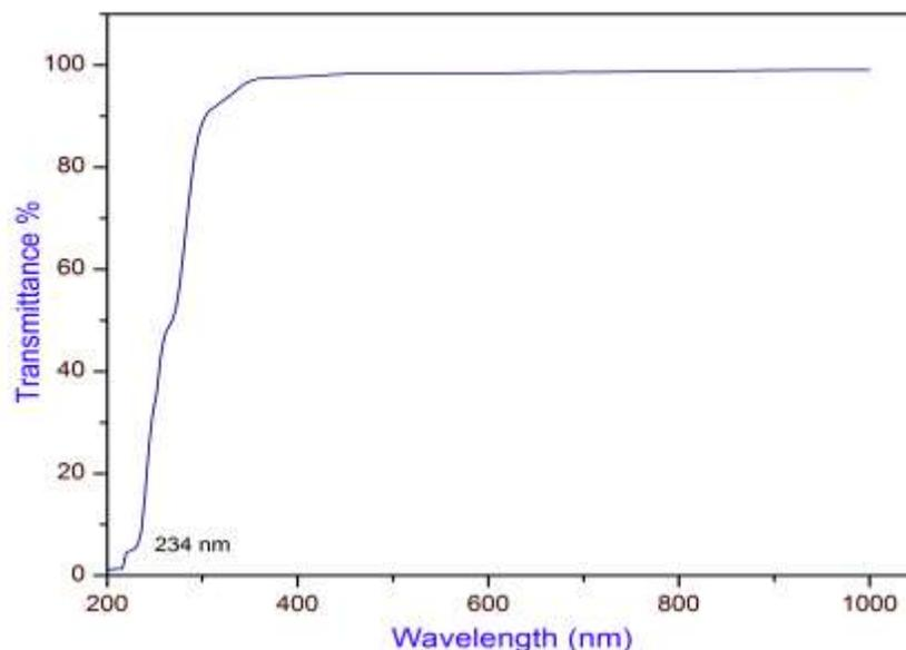
Figure 4 Optical transmission spectrum of LMC crystal
