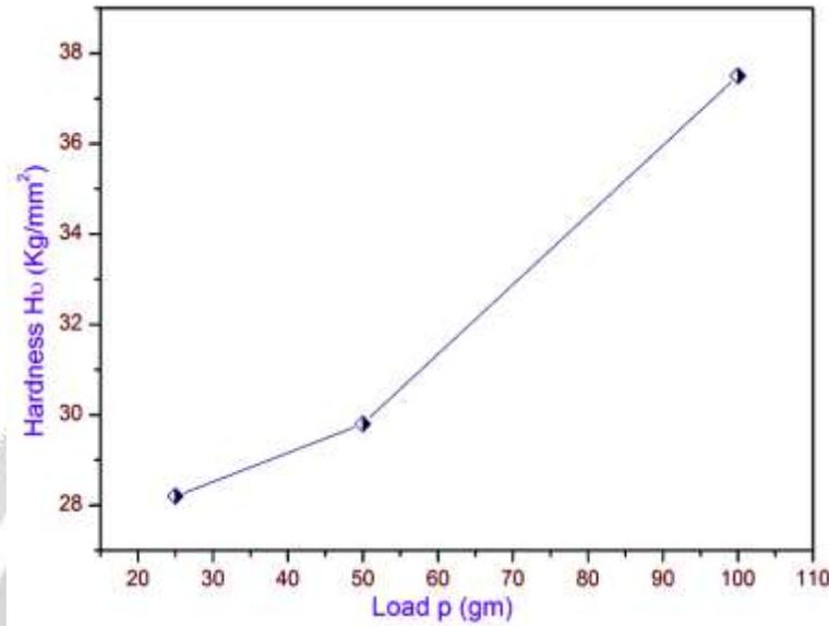
Figure 7 plot of load ( $p$ ) Vs Hardness ( $H_v$ ) for LMC crystal
