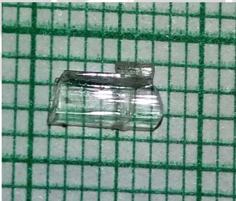
Figure 1 As grown LMC crystal
