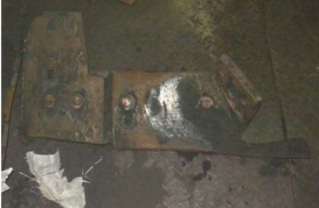
Fig 4.3.1. Worn Mixer Blade
