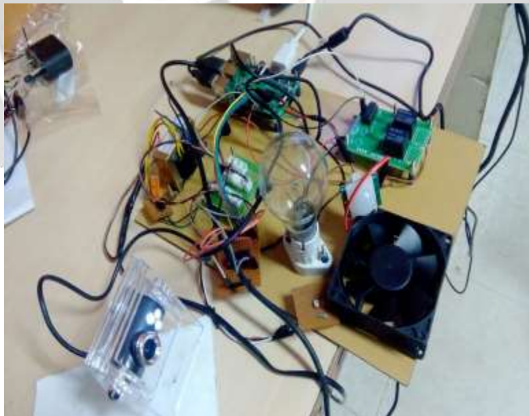
Fig -4 Prototype of Raspberry Pi based Home Automation System
