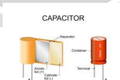
Fig9: The figure shown above is of a capacitor
