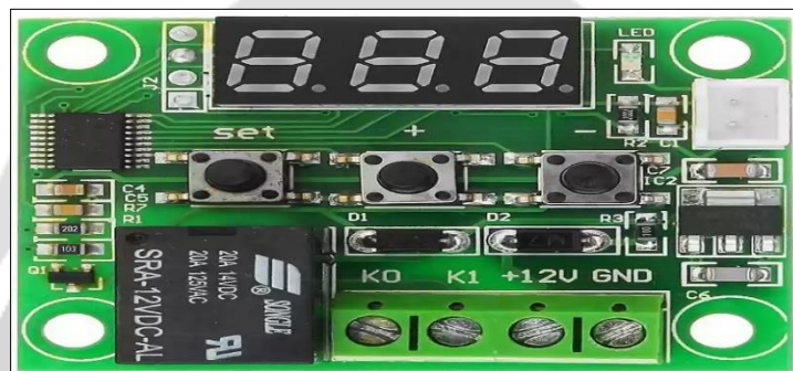
Fig 3.7 Digital temperature controller
